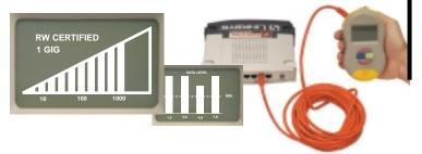
DECODE A HUB, SWITCH AND PC'S CAPABILITIES AND SIGNAL LEVEL. GO "INLINE" BETWEEN TWO DEVICES FOR THE "NEGOTIATED" SPEED.
