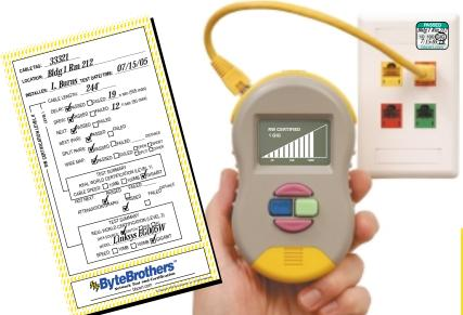
Record your test results on the enclosed tablet. Affix the enclosed "PASSED" labels to the cables and devices that have been tested.
